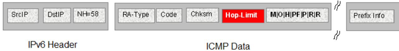
Figure 9: IPv6 ICMP RA data packet outline
