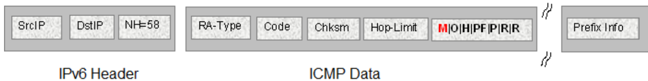
Figure 8: IPv6 ICMP RA data packet outline
