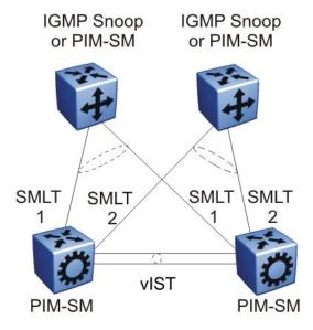
Figure 20: Multicast routing using PIM-SM
