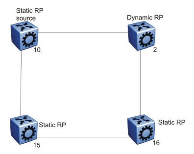
Figure 15: Unsupported static RP configuration
