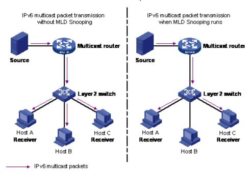
Figure 26: IPv6 multicast packet transmission when MLD snooping is enabled and not enabled
