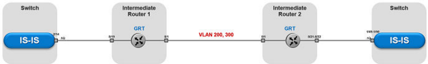
Figure 31: FE over Pseudowire traffic flow component view
