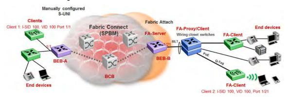
BEB-B is a switch acting as the FA Server with an NNI interface to the SPBM cloud. FA Client and FA Proxy devices send I-SID-to-VLAN mapping requests to the FA Server on the respective FA-enabled ports, using LLDP TLVs. This enables the I-SID endpoints to communicate with the SPB cloud.
