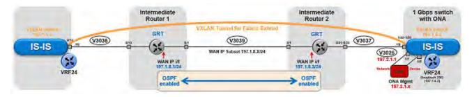
Figure 28: IP (VRF) traffic flow component view
