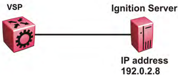
Figure 34: VSP switch connects to the Identity Engines Ignition Server
