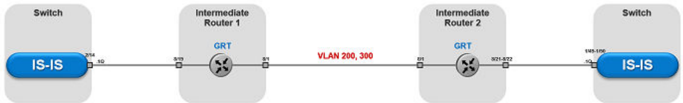
Figure 31: FE over Pseudowire traffic flow component view
