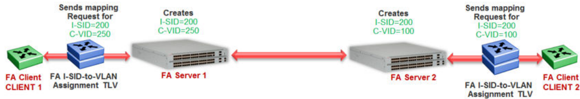
Figure 17: Learning of I-SID-to-VLAN mappings
