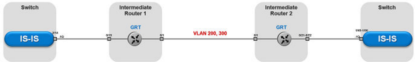
Figure 31: FE over Pseudowire traffic flow component view
