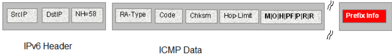
Figure 6: IPv6 ICMP RA data packet outline
