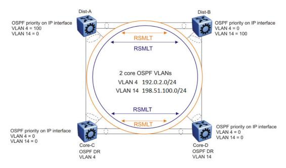
Figure 5: RSMLT with dual core VLANs
