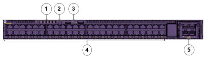
1. Mode button for port LED control. Port LED mode indicators (SYS, SPD). Switch LEDs for system power (P1, P2) and fans (F1, F2, F3). System Locator LED (LOC).
