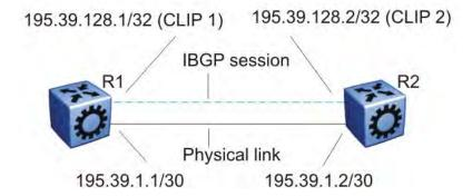
Figure 16: Routers with iBGP connections
