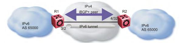
Figure 25: iBGP+ peers on CLIP interfaces with IPv6 tunneling
