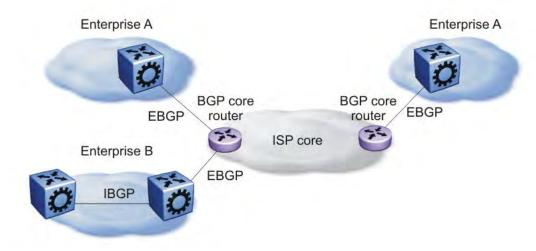
Figure 19: BGP and Edge Aggregation
