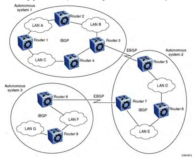
Figure 1: Internetwork segmented into three autonomous systems
