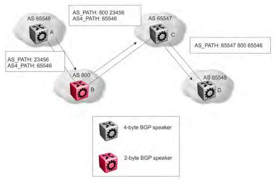
Figure 3: 2-byte and 4-byte Mixed Environment
