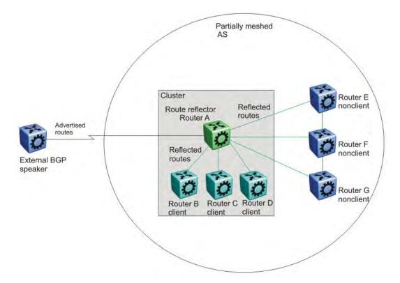
Figure 11: Route reflector with client and nonclient peers
