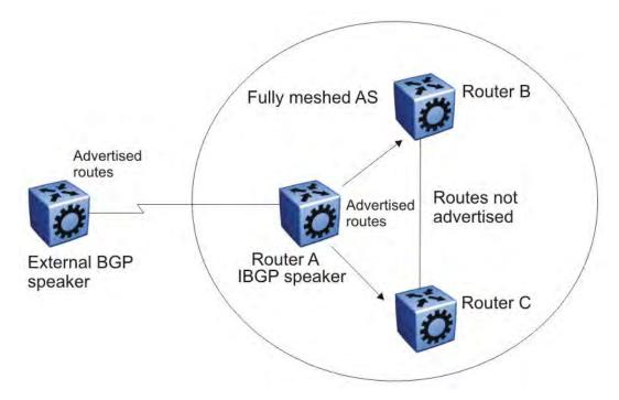
Figure 9: Fully meshed AS with iBGP speakers
