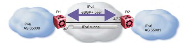
Figure 24: eBGP+ peers with IPv6 tunneling
