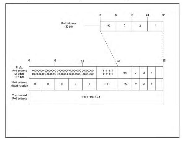
Figure 23: IPv4-mapped IPv6 address components
