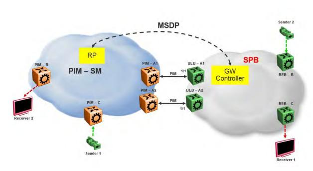
Figure 7: SPB-PIM Gateway base case configuration
