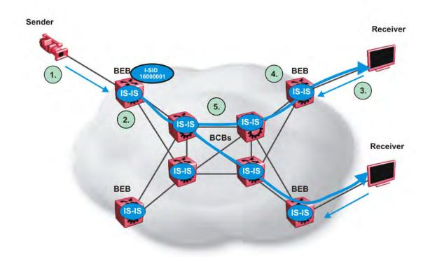
Figure 1: IP Multicast over Fabric Connect streams
