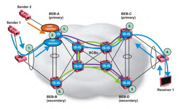
Figure 2: IP Multicast over Fabric Connect streams in an SMLT configuration
