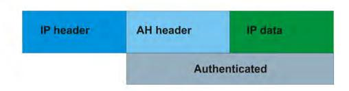
Figure 19: AH in transport mode
