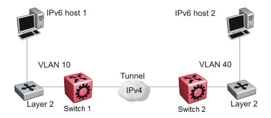
Figure 11: Tunnel configuration between brouter ports
