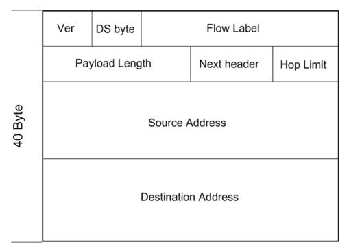
Figure 2: IPv6 header
