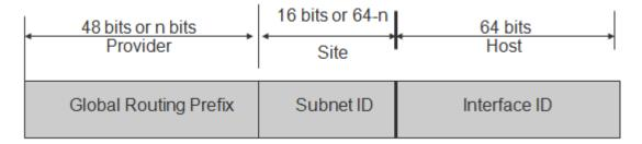
Figure 5: Unicast global address parts
