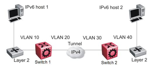
Figure 12: Tunnel configuration between VLANs
