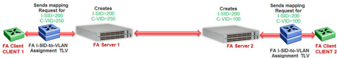
Figure 17: Learning of I-SID-to-VLAN mappings
