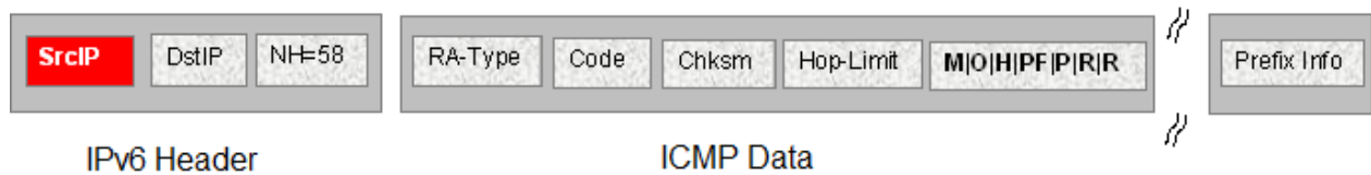
Figure 5: IPv6 ICMP RA data packet online
