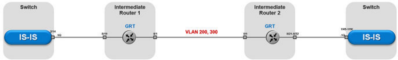
Figure 31: FE over Pseudowire traffic flow component view
