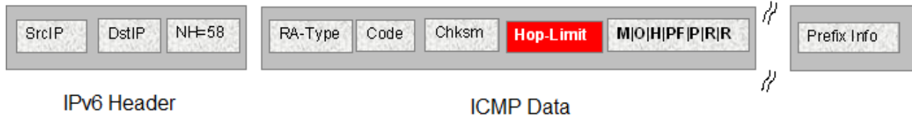
Figure 9: IPv6 ICMP RA data packet outline
