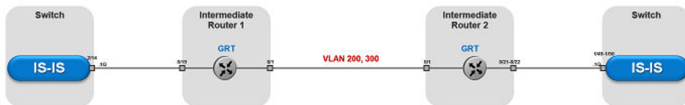
Figure 31: FE over Pseudowire traffic flow component view
