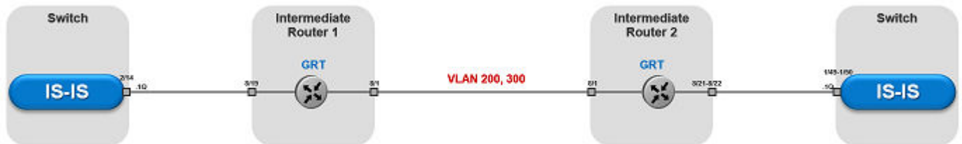
Figure 36: FE over Pseudowire traffic flow component view
