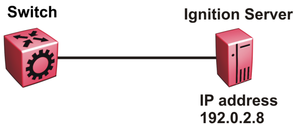
Figure 37: A switch connects to the Identity Engines Ignition Server
