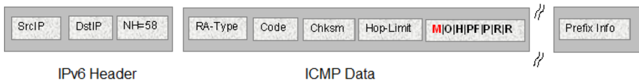
Figure 8: IPv6 ICMP RA data packet outline
