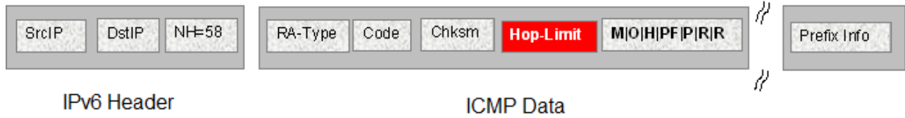
Figure 9: IPv6 ICMP RA data packet outline
