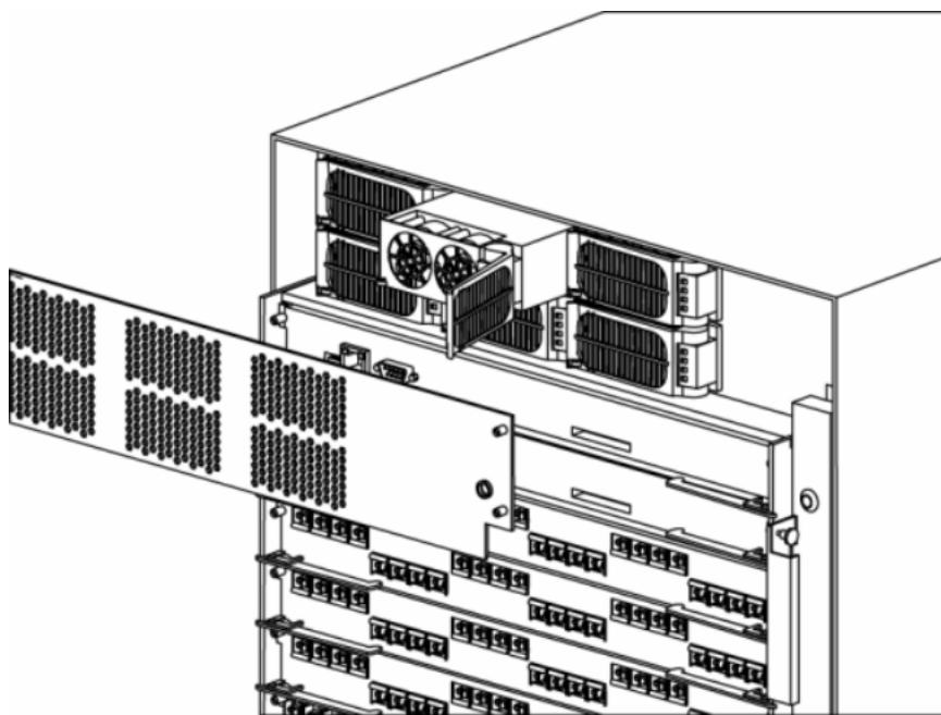
2. Push the power supply firmly into the bay until the action lever clicks.
