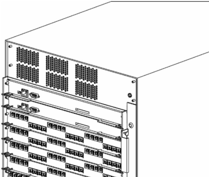
2. Pull the power supply filler panel from the chassis.
