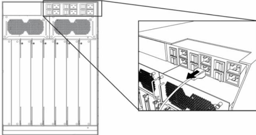
3. Pull the action lever to release the power supply.
