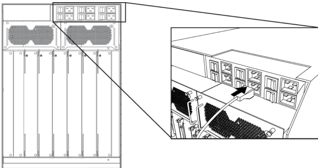
The 9006AC power supply measures 1.625 inches (in.) x 4 in. x 13.875 in. (41.3 millimeter [mm] x 101.6 mm x 352.4 mm) and weighs 5 pounds (2.27 kilograms).
