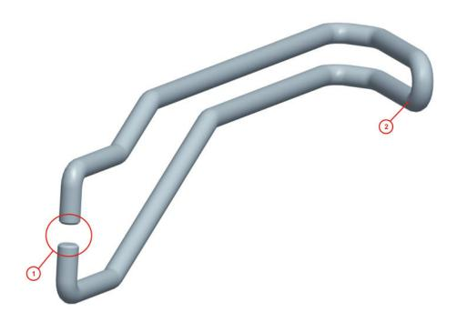
2. With the hooked end facing out, insert the dual-pronged end of the locking lever into the locks on the left side of the upper cable management bracket.
