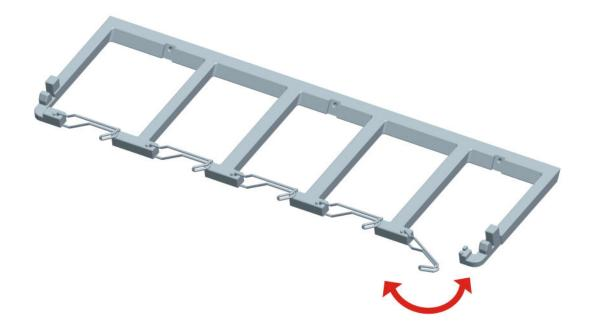
4. Grasp the hooked end of the lever to engage or disengage the locking feature, and lift the hooked end of the lever over the locking pin.
