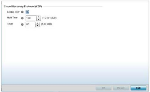
Figure 5-104 Profile Overrides - Network Cisco Discovery Protocol screen
