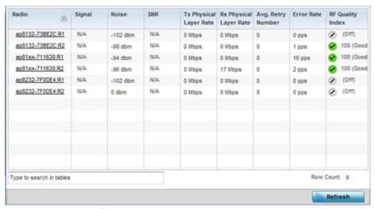
Figure 15-18 RF Domain - Radio RF Statistics screen
