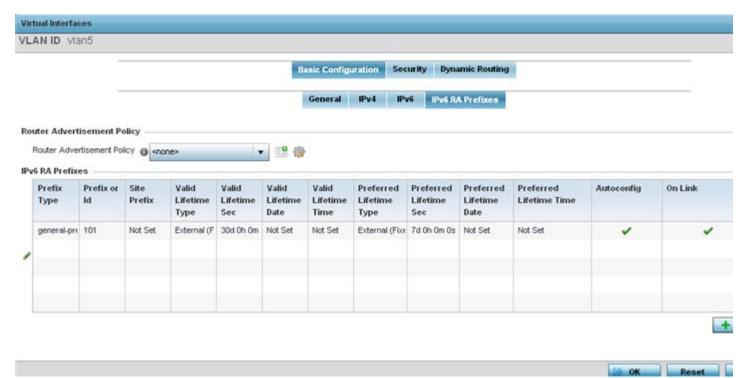
Figure 5-41 Virtual Interfaces - Basic Configuration screen - IPv6 RA Prefixes tab
