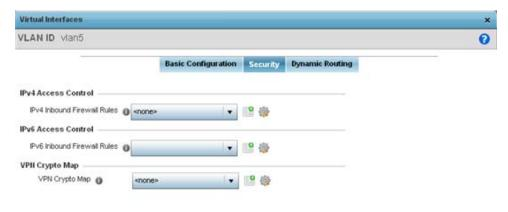
Figure 5-92 OSPF Virtual Interface - Security screen
