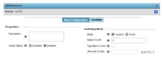
Figure 5-50 Profile Overrides - VM Interfaces Basic Configuration screen
