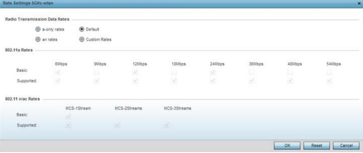
Figure 6-53 Advanced Rate Settings 5 GHz screen
