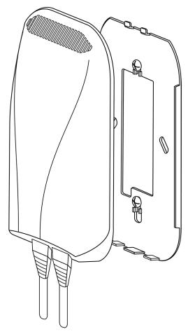
4 Cable the AP-7602 using either the Power Injector solution, an approved AP-7602 power supply or a POE enabled switch.
