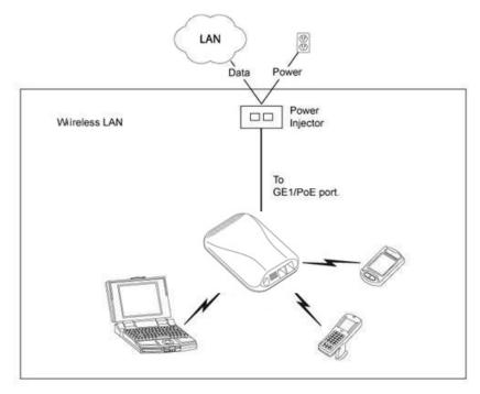
The Power Injector can be installed free standing, on an even horizontal surface or wall mounted using the power injector's wall mounting key holes. The following guidelines should be adhered to before cabling the Power Injector to an Ethernet source and an AP-7602:
