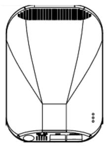
The LEDs provide a status display indicating error conditions, transmission, and network activity for the 5 GHz 802.11ac (amber) radio, 2.4 GHz 802.11n (green) radio and Bluetooth activity (blue) radio.
