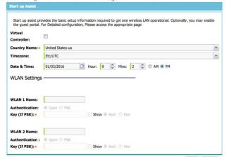
Select the Basic configuration screen, then click Startup Assist. Set the following Startup Assist parameters:
