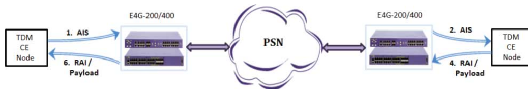
Figure 24: SAToP Alarm Handling: TDM Service AIS Alarm
