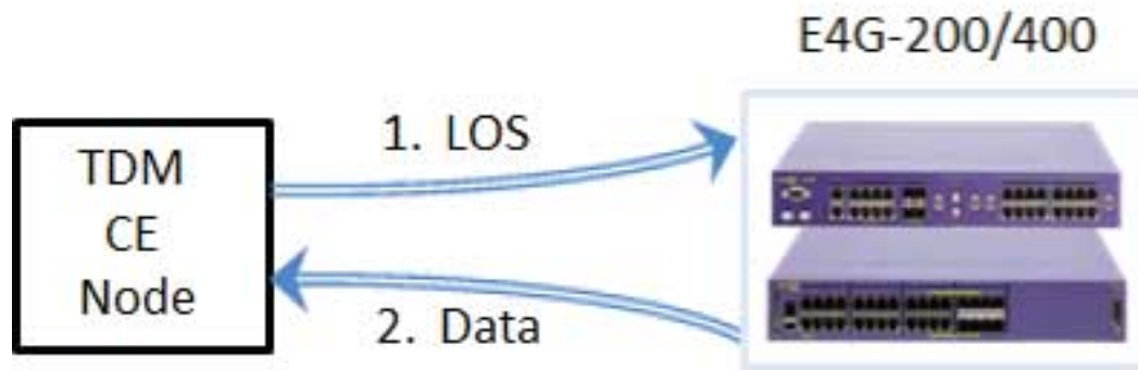
Figure 19: LOS Alarm Response
