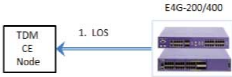
Figure 22: LOS Alarm Generation
