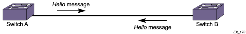
Figure 46: Extreme Networks Switches with ELSM-Enabled Ports Exchanging Hello Messages
