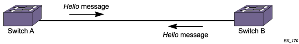
Figure 59: Extreme Networks Switches with ELSM-Enabled Ports Exchanging Hello Messages
