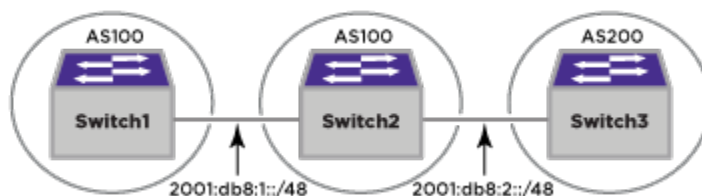
Figure 264: BGP IPv6 Example
