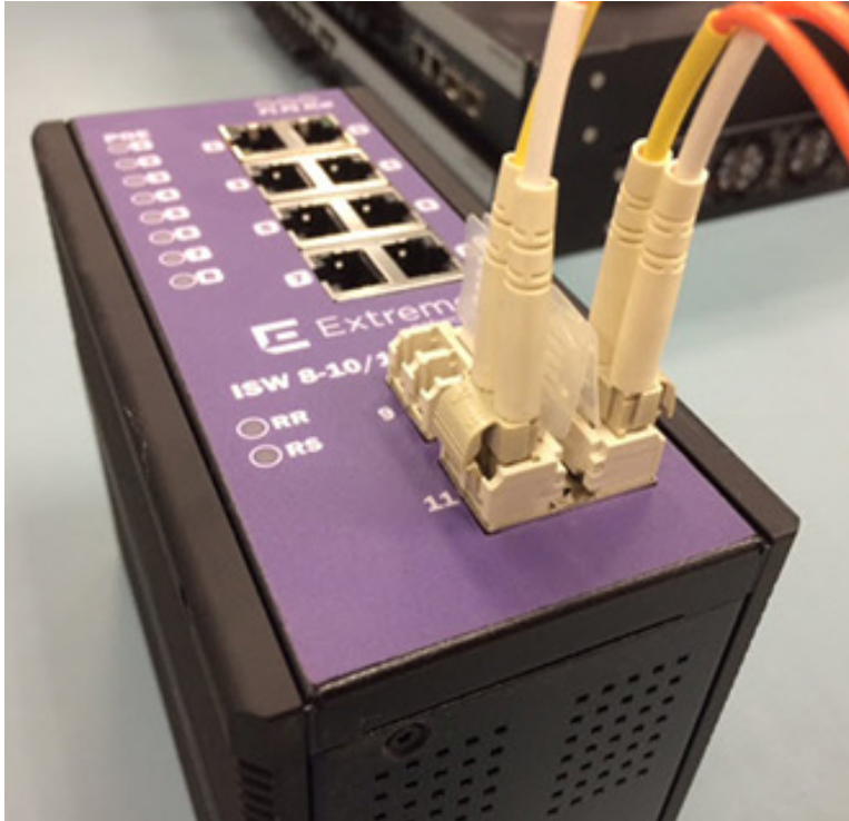
Figure 25: Connect the optical fiber to the SFP socket
