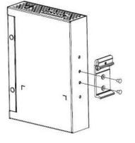
The DIN-rail bracket has a metal spring in the upper rail of the bracket. This spring is compressed for mounting and un-mounting by applying downward force.
