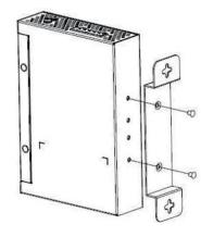
Figure 3 DIN-rail Bracket Assembly
