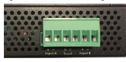
The standard screw torque for the terminal block is 3.5 kgf/cm.
