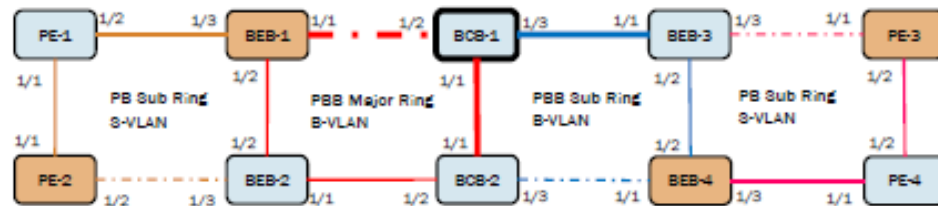
FIGURE 150 PBB interconnection node (BCB)
