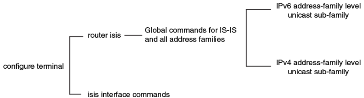
FIGURE 38 IS-IS CLI levels
