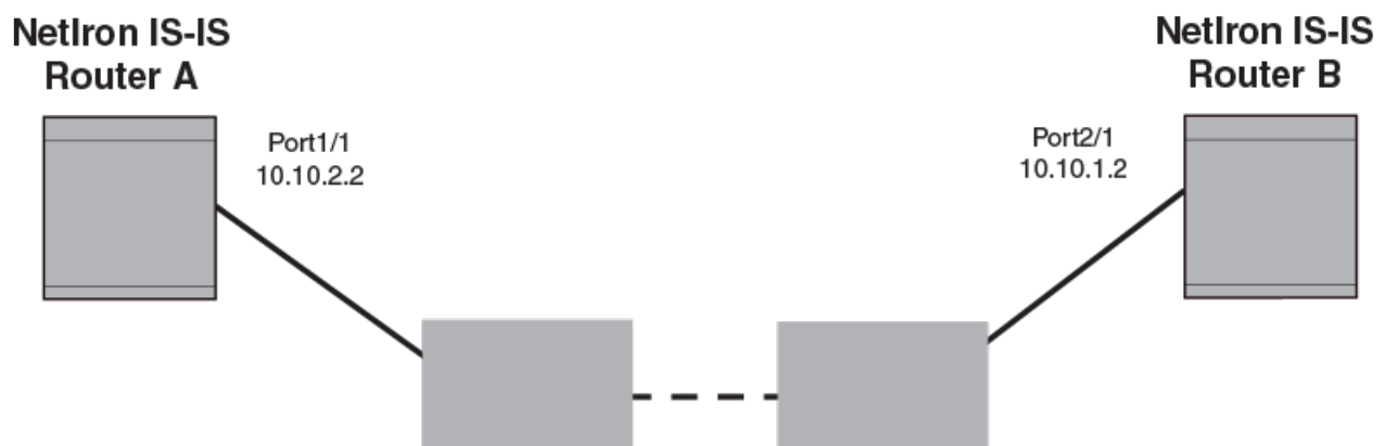
FIGURE 39 IS-IS Point-to-Point configuration
