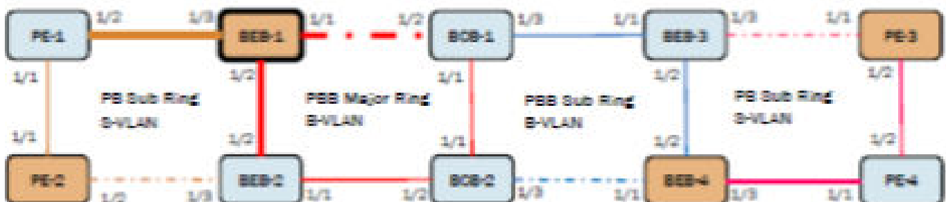
FIGURE 134 PBB interconnection node (BEB) sample configuration
