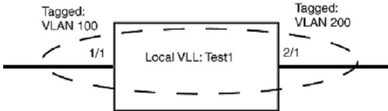
FIGURE 70 Local VLL "Test1" with two tagged VLANs
