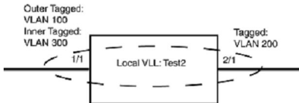
FIGURE 71 Local VLL "Test2" with one single-tagged VLAN and one dual-tagged VLAN
