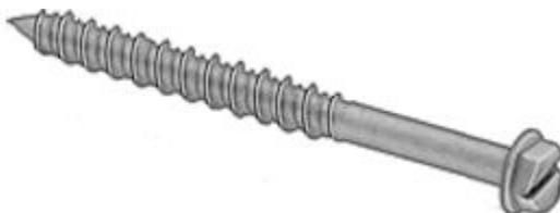
Typical drill size is 5/32" for the 3/16" concrete screw. Follow the manufacturer's instructions, including the recommendation for drill depth.
