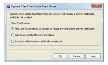
Management Center and NAC use server certificates to provide secure communication for application web pages and for internal communication between server components. When a server certificate is replaced, Management Center clients must be configured to trust the new certificate. A trust mode is used to determine how all clients handle updated certificates. You can set the client trust mode to one of the following options:
