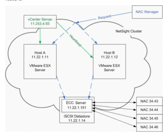
In this configuration, the vCenter Server is configured to manage the hosts in a cluster called "Management Center Cluster." There are two hosts with VMware's ESX server installed on them: Host A (11.22.1.11) and Host B (11.22.1.12). The vCenter Server is installed on a Windows server machine at 11.253.4.55. The vCenter Server is configured to send heartbeat requests to the hosts and considers them failed if it does not hear a response within 30 seconds. Both hosts are
