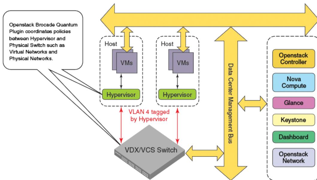
The Brocade Neutron ML2 Plugin communicates with the Brocade Mechanism Driver, which uses NETCONF on the backend to configure the Brocade switches.
