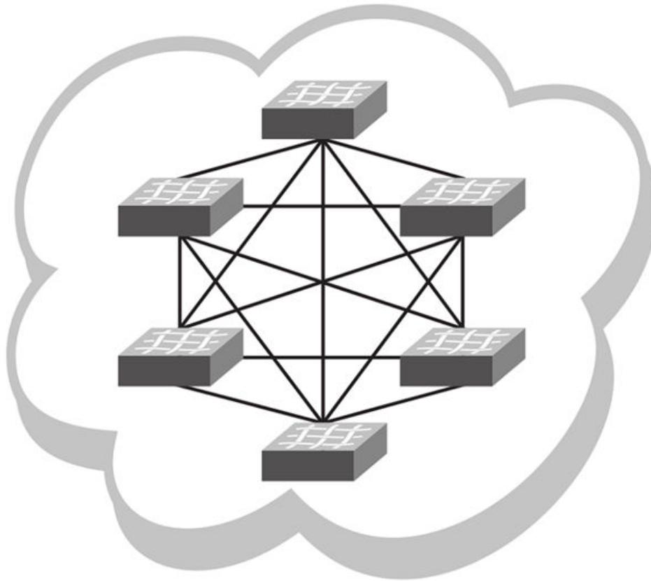
This topology is highly reliable and fast, but it does not scale well. It is reliable because it provides many paths through the fabric in case of cable or node failure. It is fast with low latency because you can get to any node in the fabric in just one hop. It does not scale well because each additional node increases the number of fabric links and switch ports exponentially. This topology is suitable for smaller fabrics only.
