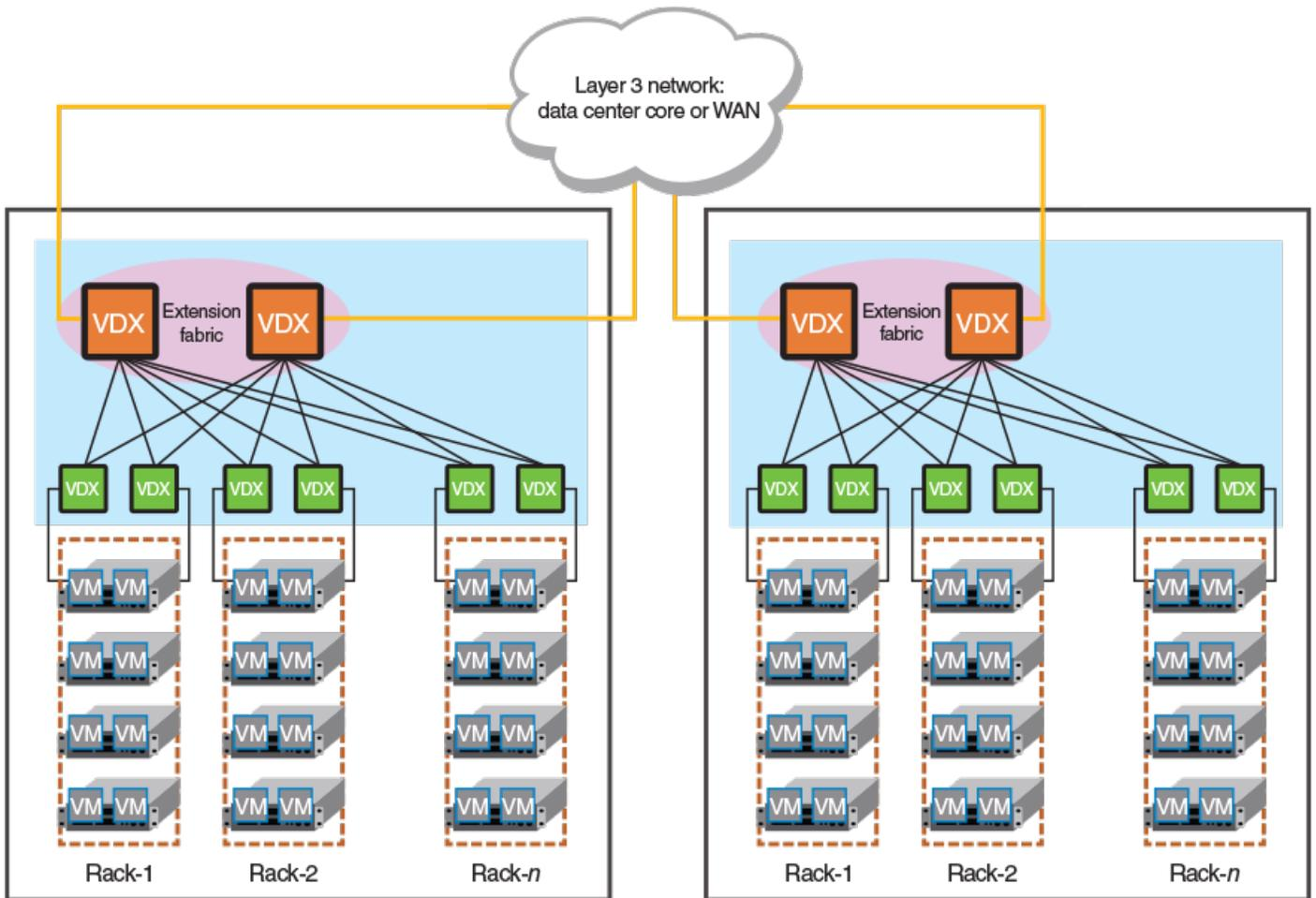
The following illustrates an example high-level topology that uses VXLAN virtual network interface (VNI) tunnel endpoints (VTEPs) in separate fabrics with a one-arm VDX deployment. Note the following restrictions for this topology:
