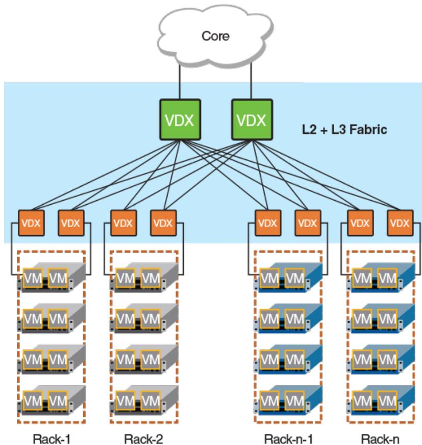
In this topology, bridging a physical server and VXLAN servers that are located in the same rack requires interaction with an aggregation gateway, introducing an extra hop. The gateway supports VXLAN Network Identifier (VNI) classification for both east-west and north-south traffic. Note the following considerations:
