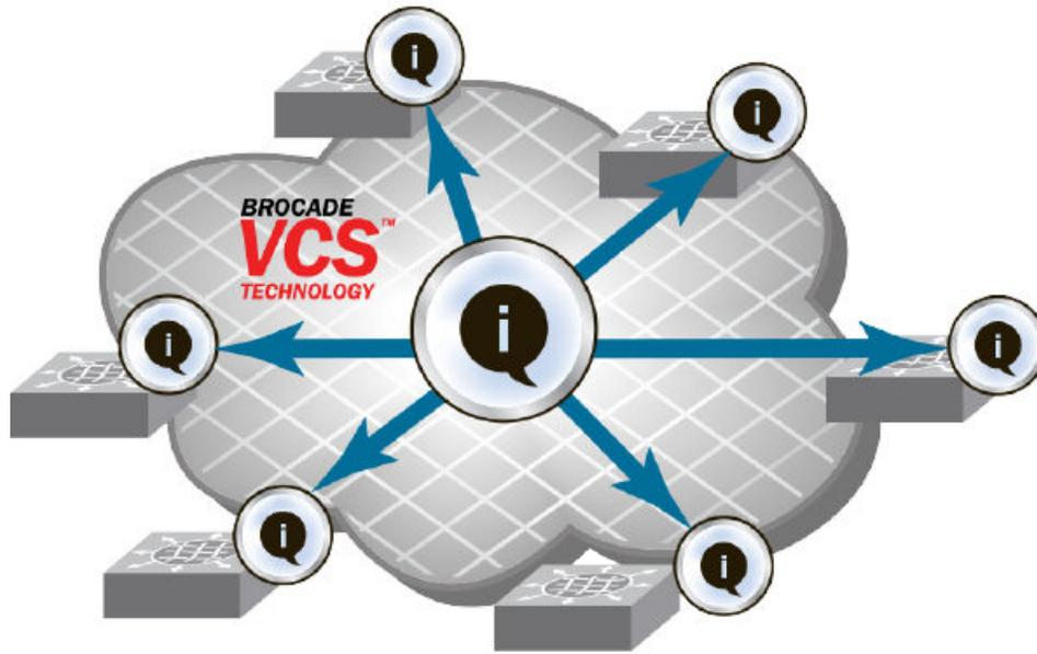
A Brocade VCS Fabric is designed to be managed as a single "logical chassis," so that each new switch inherits the configuration of the fabric, and the new ports become available immediately. The fabric then appears to the rest of the network as a single switch. This significantly reduces complexity for the management layer, which in turn improves reliability and reduces troubleshooting.
