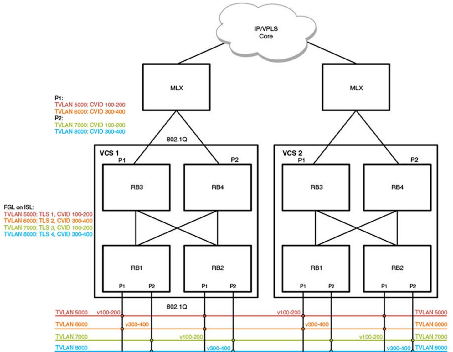
The transport VFs that can extend outside of the VCS Fabric are numbered up through 4095, bound by the 802.1Q interface. Because the extension port cannot support QinQ encapsulation, transport VFs that have overlapping C-TAGs cannot be configured on the same port. In the initial release of this feature, no Layer 2 or Layer 3 configuration is supported.
