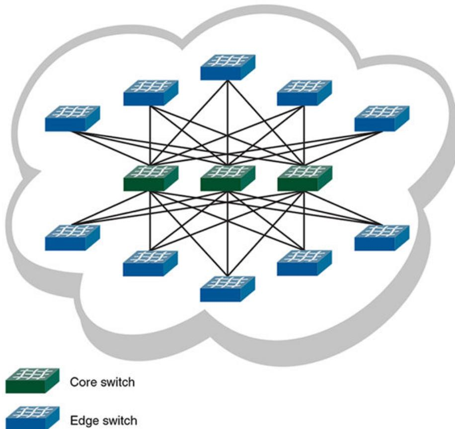
This topology is reliable, fast, and scales well. It is reliable because it has multiple core switches. If a core switch or a link to a core switch fails, an alternate path is available. As you increase the number of core switches, you also increase the number of link or core switch failures your cluster can tolerate.
