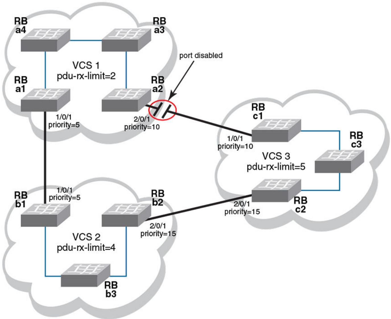
With all ELD enabled edge ports sending PDUs at the same rate, VCS1 reaches its pdu-rx-limit first. Port 2/0/1 has a lower priority (higher priority number) than port 1/0/1, and is therefore selected to be disabled. If both ports have the same priority, the port with the higher port-ID is disabled.
