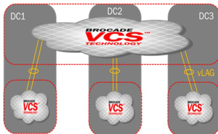
Standard VCS Fabrics scaling limitations apply if Inter-Switch Links (ISLs) are used over distances of up to 1000 m. Using Inter-Switch Links (ISLs) over longer distances (more than the standard 1000 m) is currently available for 10G, 40G, and 100G ISLs and can be done in two ways:
