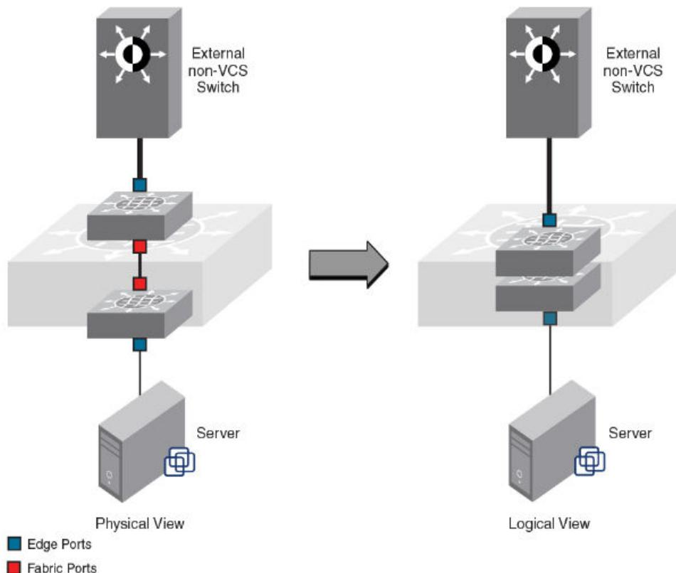
Each physical switch in the fabric is managed as if it were a blade in a chassis. When a Brocade VCS Fabric-mode enabled switch is connected to the fabric, it inherits the configuration of the fabric and the new ports become available immediately.
