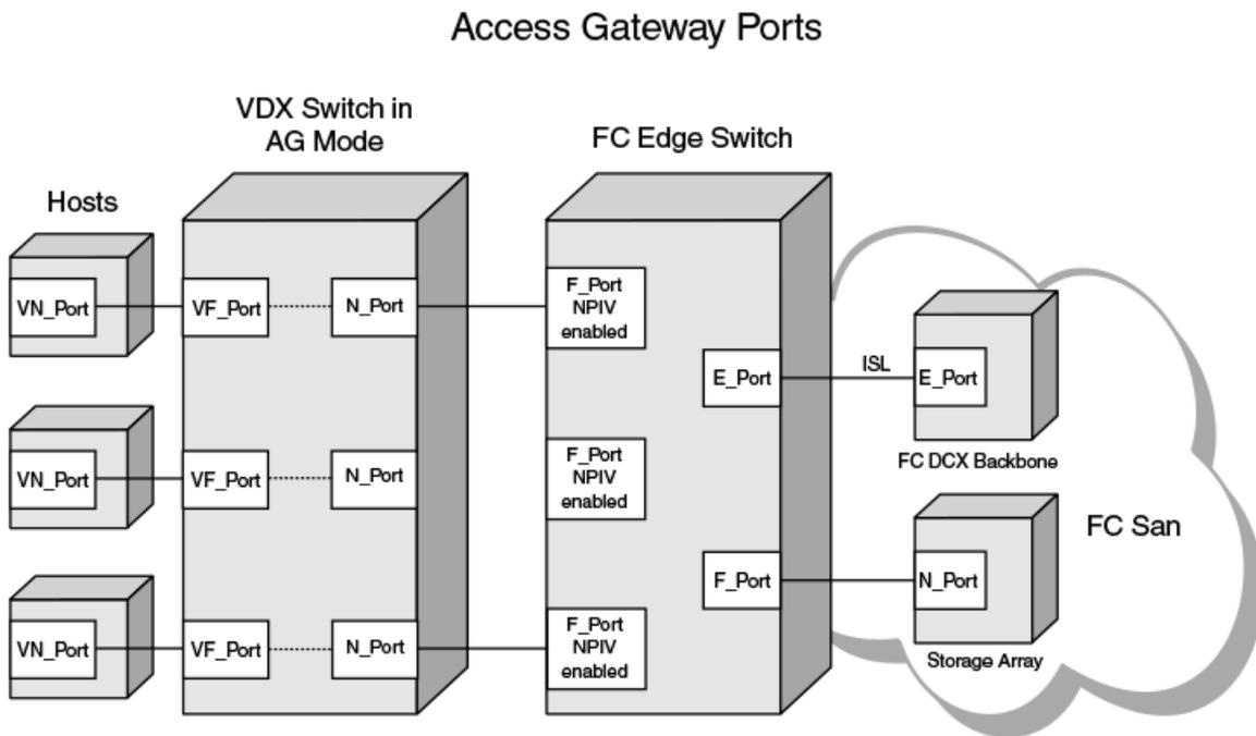
The following figure illustrates the ports used for connecting hosts attached to a non-AG (native) switch to a Fibre Channel switch, using an ISL connection.
