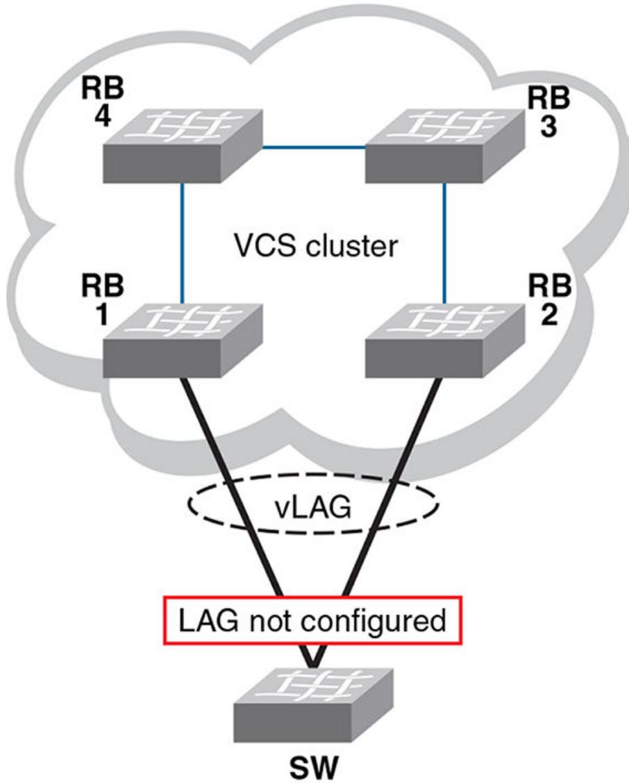
The following figure shows another example for which ELD could be used to detect and break a Layer 2 loop. In this case, multiple Brocade VCS Fabric clusters are interconnected in a manner that creates a Layer 2 loop.
