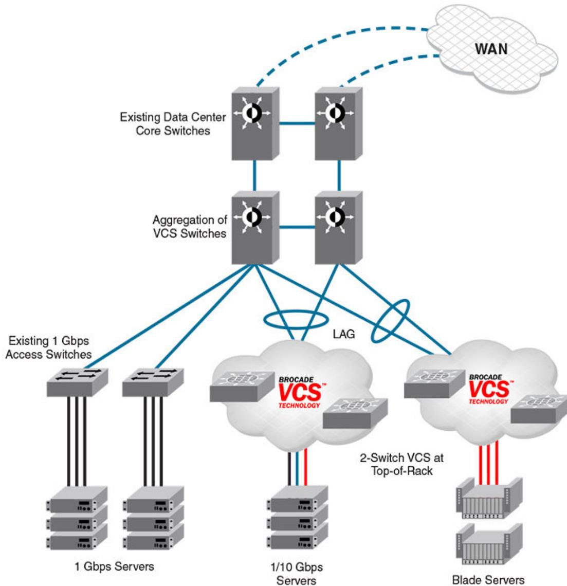
The servers perceive a single top-of-rack switch, allowing for active/active connections running end-to-end.
