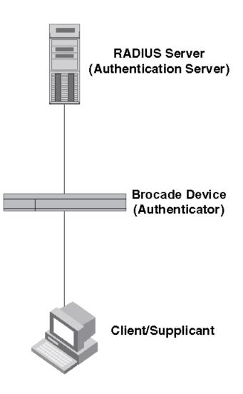
Authenticator: The device that controls access to the network. In an 802.1X configuration, the Brocade device serves as the authenticator. The authenticator passes messages between the client and the authentication server. Based on the identity information supplied by the client, and the authentication information supplied by the authentication server, the authenticator either grants or does not grant network access to the client.
