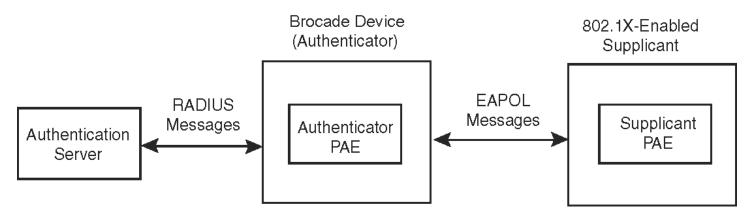
Authenticator PAE: The authenticator PAE communicates with the supplicant PAE, receiving identifying information from the supplicant. Acting as a RADIUS client, the authenticator PAE passes the supplicant information to the authentication server, which decides whether the supplicant can gain access to the port. If the supplicant passes authentication, the authenticator PAE grants it access to the port.
