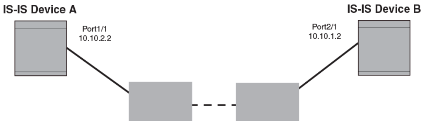
FIGURE 36 IS-IS Point-to-Point configuration
