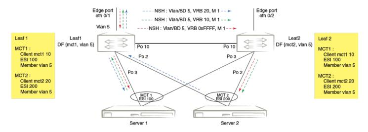
Leaf1 and Leaf2 are MCT peers. MCT1 and MCT2 are two LAGs. On both leaf nodes, MCT1 is configured with client ID 10, ESI 100 and member VLAN 5. Similarly, MCT2 is configured with client ID 20, ESI 200, and member VLAN 5. In this example, Leaf1 is DF for {ESI 100, vlan 5} and Leaf2 is DF for {ESI 200, vlan 5}.
