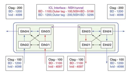
For customer 1, nodes, 1 and 2 are configured with ctag 100 on the respective eth0/1 interface. A logical interface on eth0/1 is configured for VLAN 100 and is added to BD 1100.
