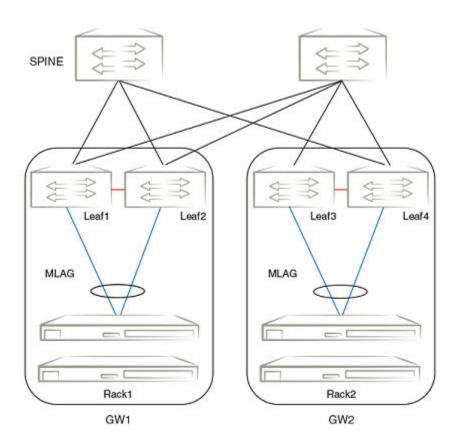
SLX-OS Layer 2 MCT is based on RFC 7432 (BGP MPLS-Based Ethernet VPN). The MP-BGP EVPN extension is the control plane on the SLX-OS device to perform both MAC synchronization and cluster management. MAC synchronization between the MCT peers synchronizes the MAC tables between the MCT nodes for node resiliency and faster convergence.
