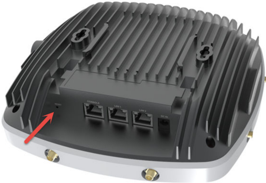
Figure 9: Position of the Reset Button on the AP3935
