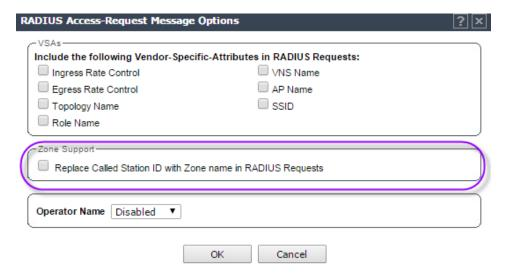
Figure 32: Configuring a WLAN Service to Send the Zone Label
