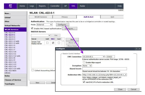
Figure 14: Configuring the Example WLAN Service for External Captive Portal
