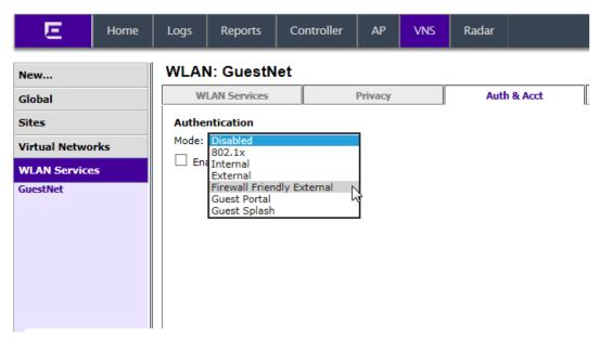
Figure 18: Selecting the "Firewall Friendly External" Support Option
