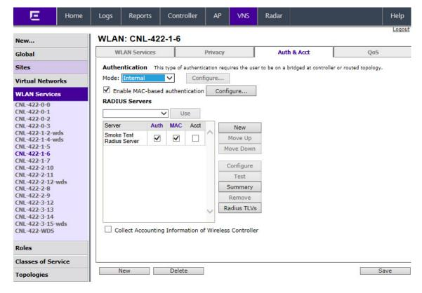
Figure 28: Configuring a WLAN Service for RADIUS Password-based Authentication
