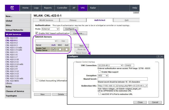
Figure 16: Configuring a WLAN Service for ECPIA (Release 9.01)
