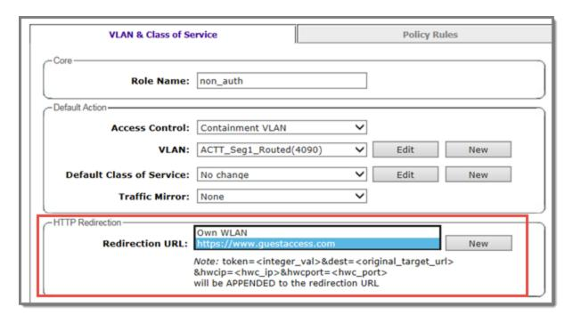
Figure 7: Example Role with Redirection specified.
