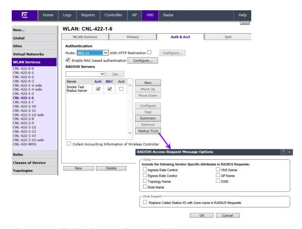
Figure 30: Configuring the Controller to Send Siemens VSAs
