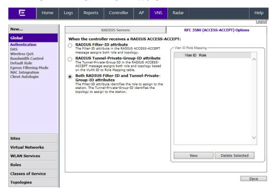
Figure 34: Configuring How the Tunnel-Private-Group-ID and Filter-Id are used
