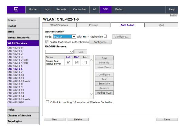
Figure 29: Configuring Wireless for EAP-based Authentication
