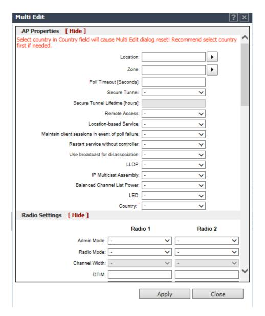
Figure 31: Assigning Zone Labels to APs Using Multi-edit
