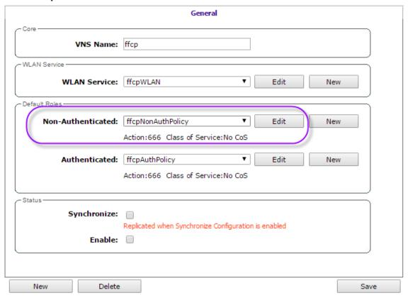
Figure 13: A VNS that Assigns the Restrictive Role to Unauthenticated Stations
