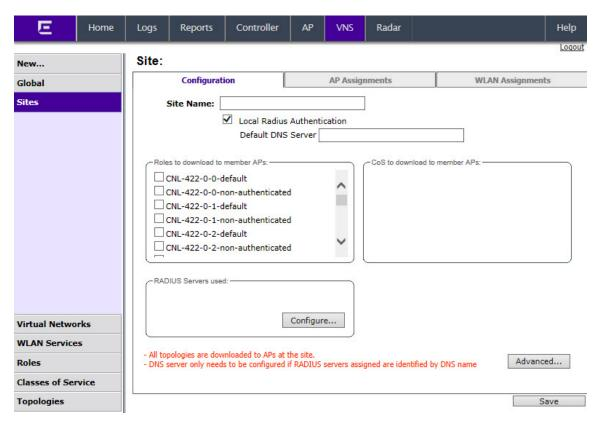
Figure 27: Configuring a Site for AP-based Authentication
