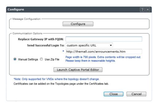
Figure 36: Configuring a WLAN Service to Redirect Successfully Logged In Users to a Specific Page
