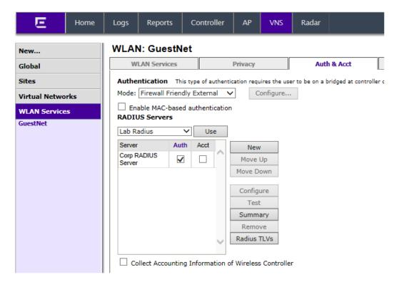
Figure 19: Configuring the RADIUS server to use for authentication
