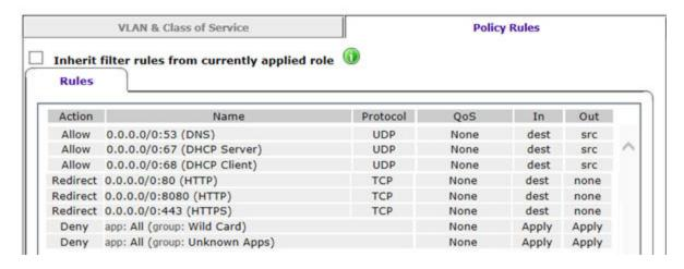
Figure 12: Rule-based Redirection for External Captive Portal
