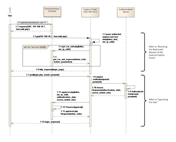
Figure 11: Flow of External Captive Portal with External Authorization
