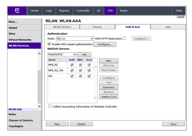
Figure 40: RADIUS Server Redundancy: Up to three usage types per server and up to three servers per usage type.
