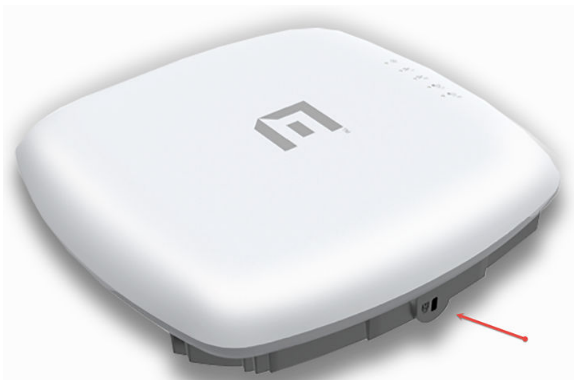
Figure 5: Kensington Lock slot
