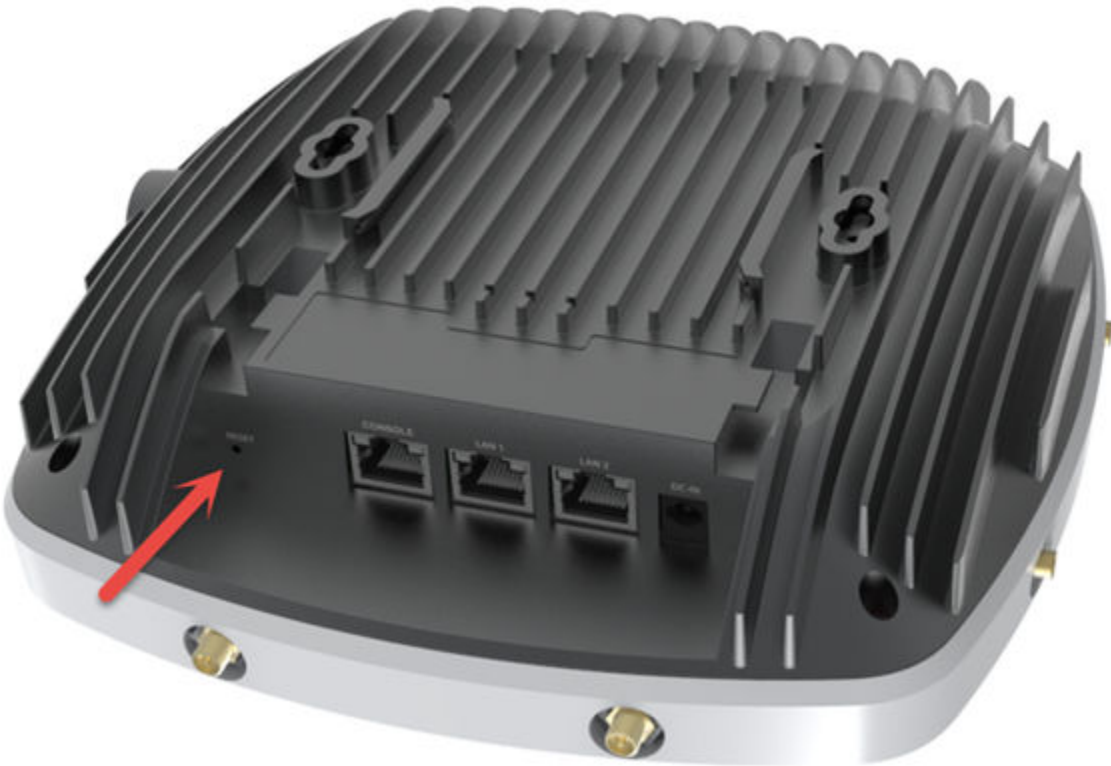
Figure 13: Position of the Reset Button on the AP3935
