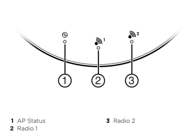
Green LEDs mean ON. Amber LEDs mean OFF.
