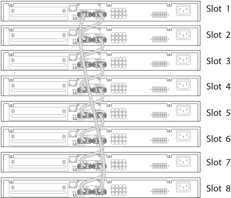
Figure 27: SummitStack Cable Connections Using Eight Switches with Integrated SummitStack Ports
