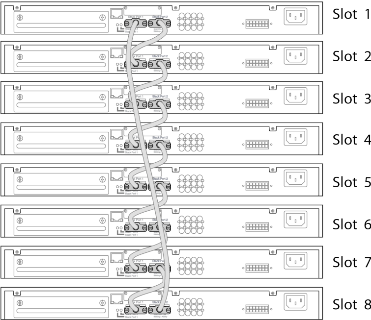
Figure 21: SummitStack Cable Connections Using Eight Switches with Integrated SummitStack Ports
