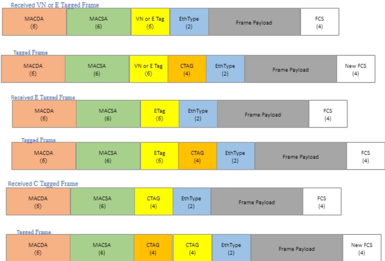
Figure 8: Tag addition, E-tag, VN-tag and C-tag frames
